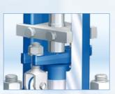
Gland packing / gland seal stuffing box provides an additional stem
