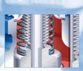
Dual function – can be used simultaneously as a check and stop valve with a tight shut-off feature due to the screw-down non-return plug with resetting spring
